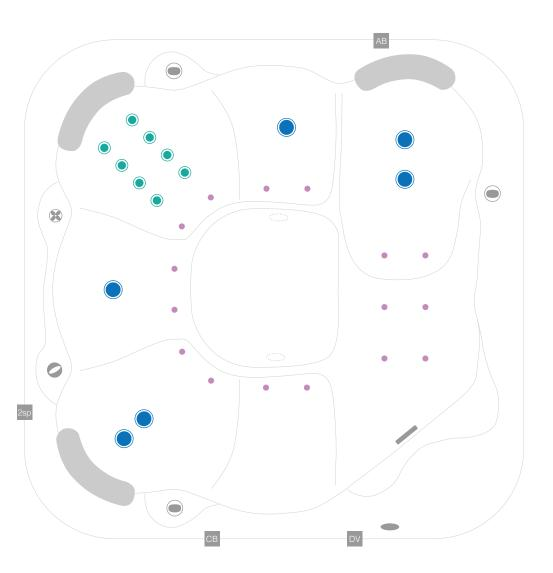
C sapphire spas. 500 series jet 400 series jet 300 series jet 200 series jet volcano jet 7" cohuna jet swim jet neck jet air massage jet  $\frown$ large divertor control small on/off control air control aromatherapy canister touchpad control filter box safety suction water return jet water spout EQUIPMENT INSTALLED IN CABINET СВ main control box filtration pump hydrojet boost pump varidrive80 pump air blower
