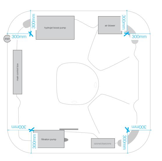
LOCATION FOR PRE-POWER THROUGH SLAB (power supply in conduit or flex to be installed in concrete slab at a MAXIMUM of 40mm above slab height)
