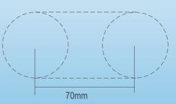
Oval and rectangle touch pad hole cutout 2 x holes cut with 65mm hole saw at 70mm centres.
