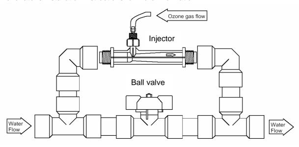
The best use of any generated ozone gas, is to dissolve it into the water and try to keep it dissolved in the water as long as possible.
