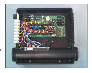
Disconnect the heater tube wiring using a pair of pliers to grip each terminal in turn—don't pull on the wire itself. Disconnect the two wires from the thermal cut out, disconnect the earth wire, disconnect the element phase and neutral wires and unplug the water sensor and temperature sensor. Unscrew the two mounting screws that locate the heater tube in place so that it can be removed.
