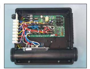
Inside every SP1200 is a 3.5, 4.5 or 6.0kW flouropolymer coated dual leg element, two over temperature cut-out devices, temperature sensor, water sensor, and a controller circuit board. To install the unit, a power supply and digital switch are needed along with a suitable pump to circulate water through the heater.
