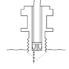
When the tip of the optical bolt is surrounded by air the light emitted by the light source is reflected back to the light detector as the tip acts like a mirror.
