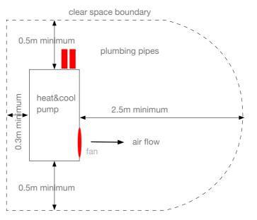
air space requirements for heat&cool pump approximate dimensions: L1000mm x W400mm x H600mm
