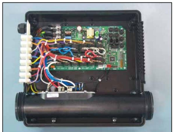
Disconnect the heater tube wiring using a pair of pliers to grip each terminal in turn—don't pull on the wire itself. Disconnect the two wires from the thermal cut out, disconnect the earth wire, disconnect the element phase and neutral wires and unplug the water sensor and temperature sensor. Unscrew the two mounting screws that locate the heater tube in place so that it can be removed.
